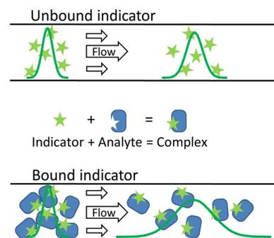
**Figure 1.** The FIDA principle is based on measuring the change in the apparent size (diffusivity) of an indicator (specific ligand) interacting with the analyte. The apparent indicator size is measured in a hydrodynamic flow system by Taylor dispersion analysis.
