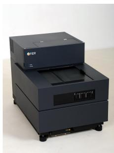
**Figure 2.** The dedicated FIDA instrument is fully automated, and has in-built assay evaluation tools. The FIDA analyser accepts vials and 96 well plates.
