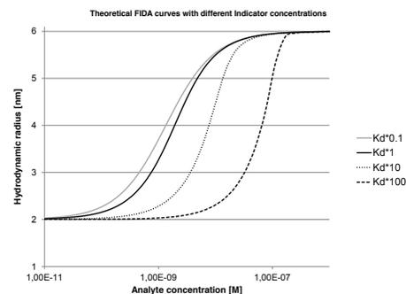
**Figure 4.** Theoretical binding curves calculated using FIDA software for different values of indicator concentration. The software allows *in silico* assay development resulting in fast assay development with limited experimental optimization.
