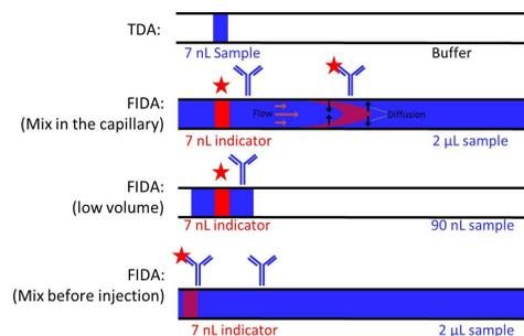
**Figure 3.** Injection and mixing procedure in the FIDA assay. Each step is fully automated using dedicated instrumentation.
